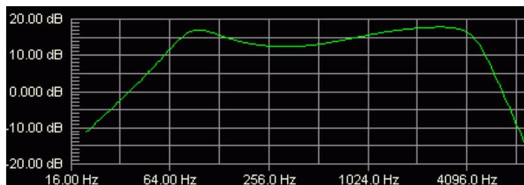
Cabsim used in **JMP-1** preamp - [schematic](#) and its frequency response:
