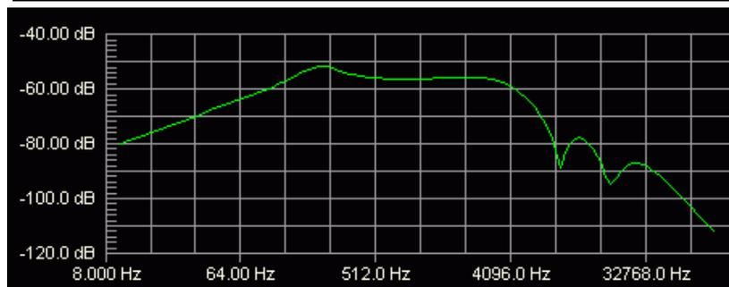
However, speaker cabinet's frequency response does not consist only of high and low frequency reduction and speaker's resonant frequency boost. In between we will find lots of "peaks" and "notches", which are results of many factors like: speaker type, speaker enclosure mechanics, or - very importantly - the cabinet surrounding. The actual frequency
