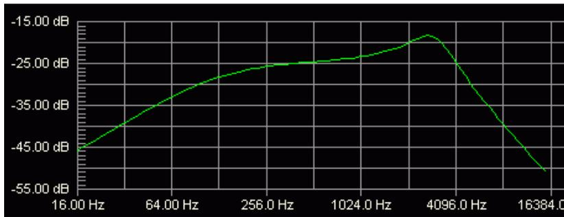
A very simple solution based on two multi-feedback filters and with an unconventional frequency response, was used in the Screamer50 amp by **ENGL**. Signal is collected after the output transformer. However, it is worth to mention that the solution does not sound perfect.
