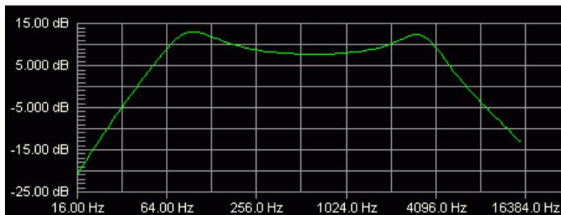
The next preamp by Mesa Boogie - **V-Twin** - has a simple filter, which can deliver purring blues tones. As usual for Mesa, the filter is based on inductance. Its [schematic](#), [sound sample](#), and frequency response:
