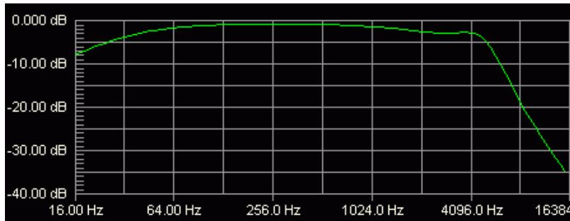
One step further; if we examine the frequency response of a guitar cabinet, we will notice another important feature - low frequency roll off starting usually at 100-200 Hz. This is achieved by using a high pass filter. Many amps contain various devices based on these two filters. Few examples - again by **H&K** - are cabinet simulators available in discontinued preamp series: **Cream Machine**, **Crunch Master**, **Metal Master** - [schematic](#) and frequency response:
